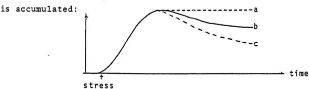
Curve <u>a</u> represents a totally unresolved stress residual, while <u>b</u> and <u>c</u> are partially accumulated.
